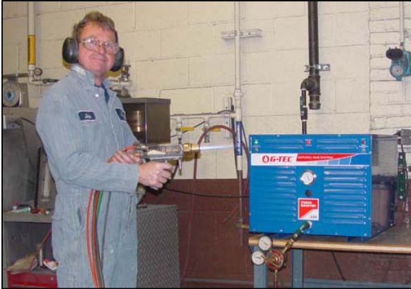
John Cooper at ASB Industries in Barberton, OH adjusts a Diamond Jet HVOF gun fueled by a G-TEC Torch Booster
