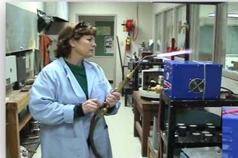
Instructor Shannon Calloway prepares to cast with hi-pressure natural gas from a TB-30 Safe-T-Gas Torch Booster at the Texas Institute of Jewelry Technology.
