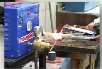
Instructor Shannon Calloway prepares to cast with hi-pressure natural gas from a TB-30 Safe-T-Gas Torch Booster at the Texas Institute of Jewelry Technology.
